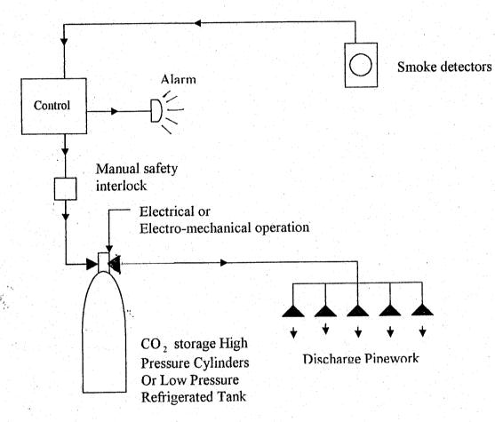
FIG. 3.5: Layout of a CO<sub>2</sub> sprinkler system.
