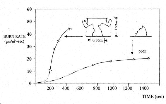
FIG. 3.0: Effect of enclosure on the burning rate of a square polymethyl methacrylate slab.
