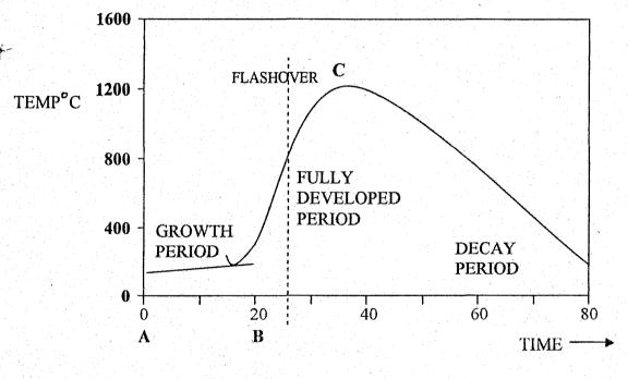
FIG.3.1: Time/temperature fire profile.
