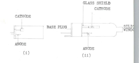
Fig. 2.2 Schematic diagram of a lamp.
