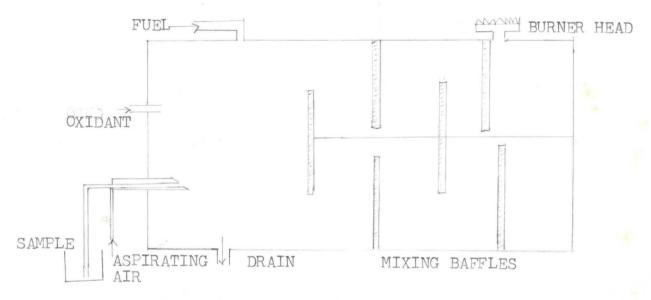
Fig.2.1 Laminar Flow; premix for Atomic Absorption
