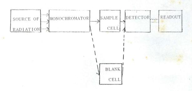
Fig. 1.0: A block diagram of the essential components of
