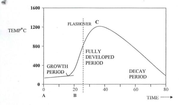
FIG.3.1: Time/temperature fire profile.
