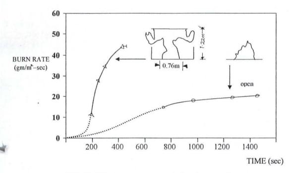
FIG. 3.0: Effect of enclosure on the burning rate of a square polymethyl methacrylate slab.
