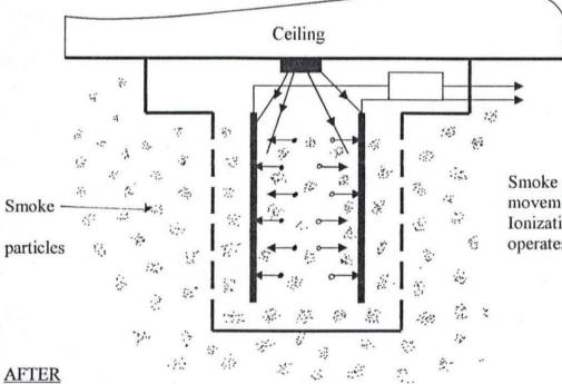
Smoke particles obstruct ion movement and reduce Ionization current - Alarm operates.
