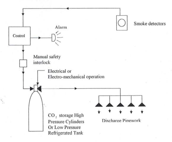
FIG. 3.5: Layout of a CO<sub>2</sub> sprinkler system.
