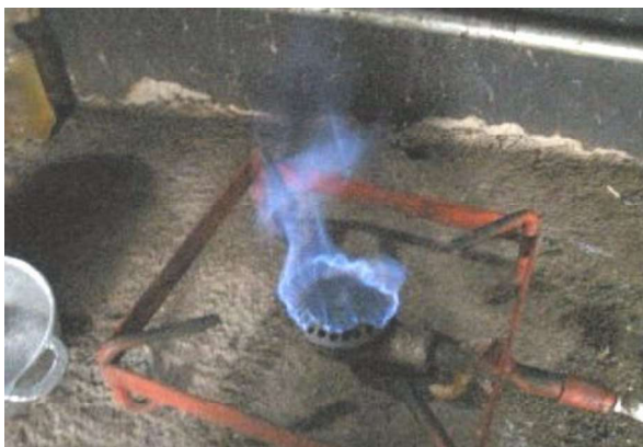
Figure 1: A typical stove burning with Biogas.
