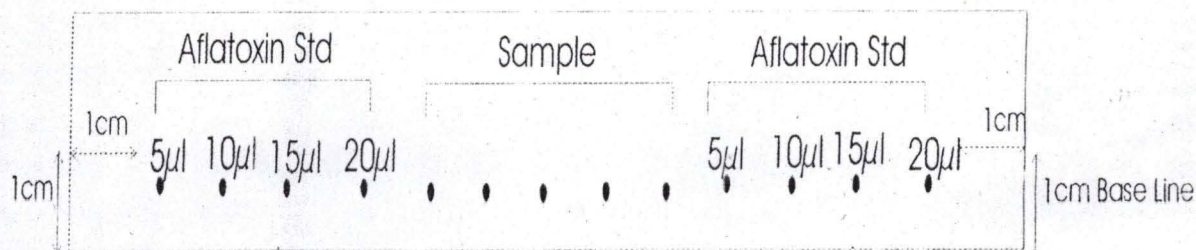
Fig4. Schematic representation of spots on chromatographic plates
