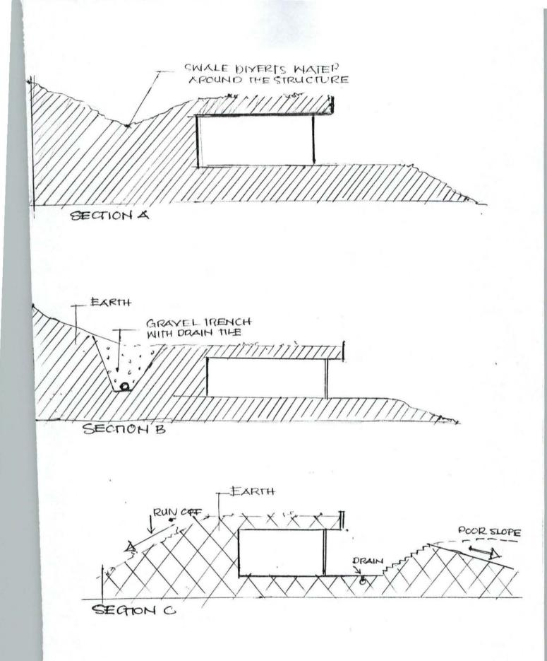
while Section B shows a cut-off gravel trench with drain tile at the base. Section C illustrates some drainage problems associated with sunken courtyards which are common in earth sheltered designs. It is preferable for the surrounding ground to slope away from the structure on all sides, then only the rainfall which falls directly into the court must be handled by a drainage system.
