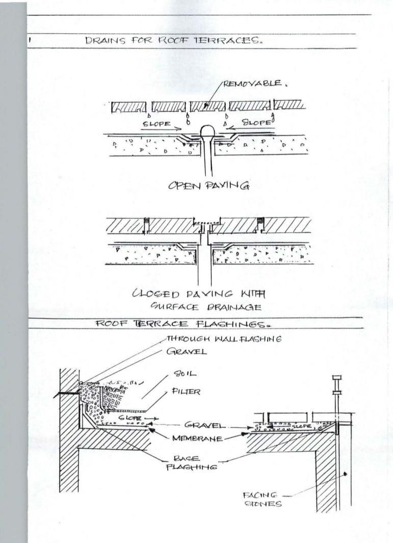
More so, the details are important to the success of a roof terrace, and in some instances the walls of the building as well. Typical schematic details are shown in figure below where the membrane is arranged to carry water away from the walls.
