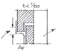
(C) WIND DRESSURE (F) WIND PRESSURE CAPILLARITY
