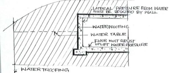
proofing technique would be needed to stop any capillary draw moisture into the wall. When temporary pressure cannot be eliminated, and this could rarely be guaranteed, damp-proofing will not surface for complete protection because damp-proofing is not designed to keep out water under pressure. Diagrams below show in the best language of architecture, what need to be done.
