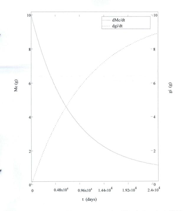
Figure 4.3: Mass of Metal and Weight Loss of Metal and Time for Corrosion in KRPC Cooling Water Pipeline at constant T = 333K;  $F_o = 1.9462$ ;  $F_s = 1.5$ ; and  $P_{CO2} = 0.5$  respectively.
