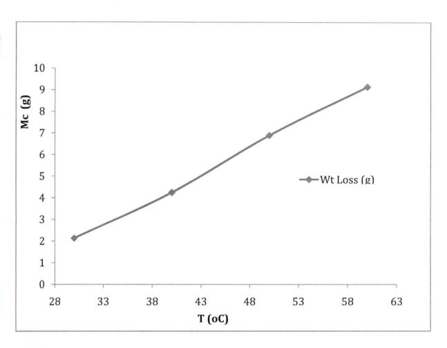
Figure 4.4: Variation of Weight Loss of Metal and Temperature for Corrosion in Cooling Water Pipeline at constant Fo = 1.9462; and Fs = 1.5; pH = 6.6 and  $P_{CO2} = 0.5$  respectively.
