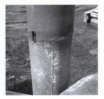
Plate xi. Uniform Corrosion on oil well pipe. (www.corrosion-club.com)
