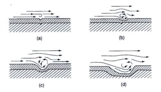
Fig.2 11 Schematic of turbulent eddy mechanism for downstream undercutting of erosion-corrosion pits
