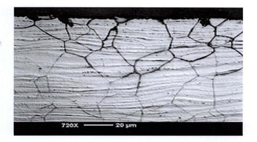
Figure 2.9: Microscope view of a polished cross section of a material attacked by intergranular corrosion (www.wikipedia.org).
