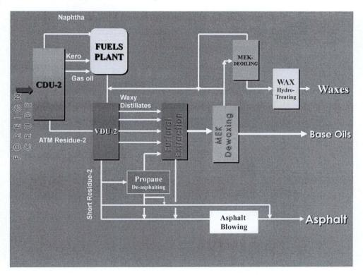
Fig.2.4 Schematic Flow Diagram of a Lube Plant. (Egbe, 2008)
