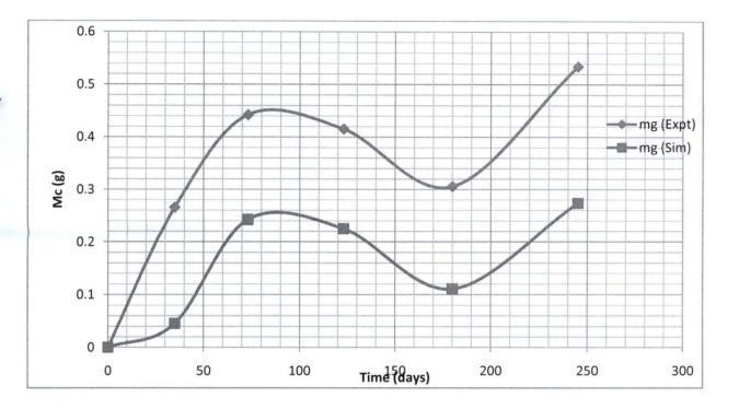
Figure 4.2: A graph of Weight Loss of Metal versus Time for Corrosion in KRPC Cooling Tower Water Return Line at Temperature of 333K.
