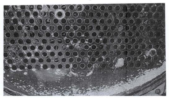
Plate ix: Heat exchanger showing pitting corrosion. (Source: Shell Global Solutions, SGS. The Hague, Netherlands).
