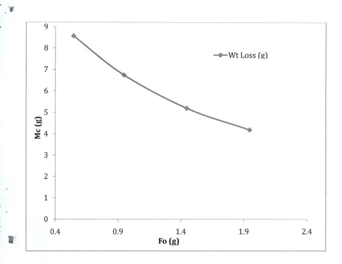
Figure 4.5: Variation of Weight Loss of Metal and Corrosion scale at 240days for Corrosion in Cooling Water Pipeline at constant T = 333K; Fs = 1.5; pH = 6.6 and P<sub>CO2</sub> = 0.5 respectively
