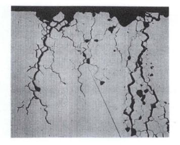
Polythionic stress corrosion cracking in Sensitised Austenitic Stainless Steel
