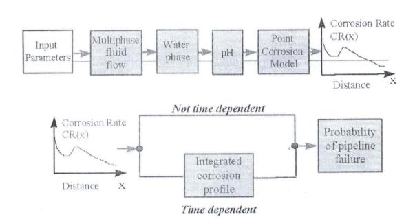
Fig: 2.16 Flow chart of the pipeline corrosion model
