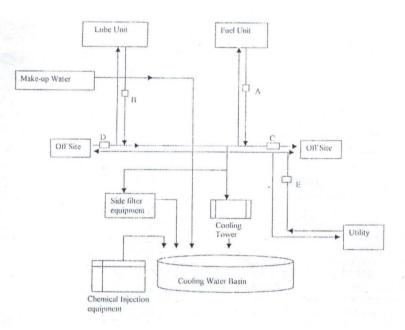
Fig.2.13 Schematic diagram showing the points of coupon installation along the cooling water pipeline. (Odigure et al, 2002)
