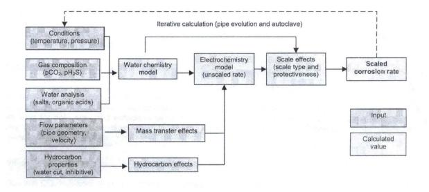
Fig: 2.15 Schematic depicting the calculation methodology of CorrCast. (Wei et al, 2009).
