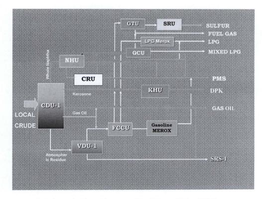
Fig. 2.2 Schematic Flow Diagram of Fuel Plant. (Egbe, 2008)
