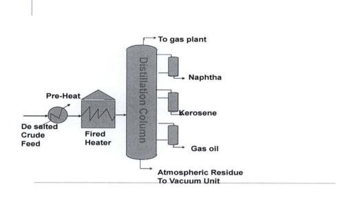
Fig.2.1 Basic Crude Distillation Unit (www.krpc.org)
