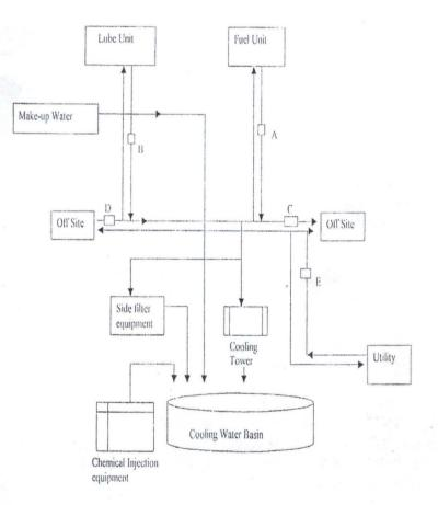
Fig.2.17 Schematic diagram showing pipeline as shown below: the points of coupon installation along the cooling water pipeline. (Odigure et al, 2002)
