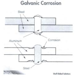
Fig. 2.7 Galvanic corrosion. (source: Shell Global solution, 2000)
