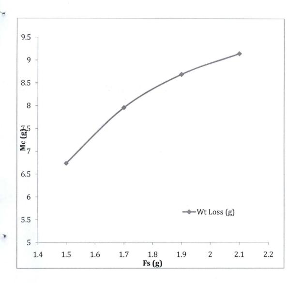
Figure 4.6: Variation of Weight Loss of Metal and Mineral Factor (Fe II content) at 240 days for Corrosion in Cooling Water Pipeline at constant T = 333K; Fo = 1.9462; pH = 6.6 and P<sub>CO2</sub> = 0.5 respectively.
