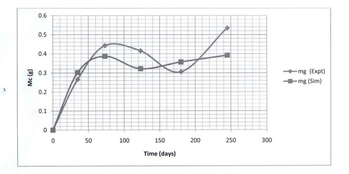
Figure 4.1: A graph of Weight Loss of Metal versus Time for Corrosion in KRPC Cooling Water Pipeline at Temperature of 333K.
