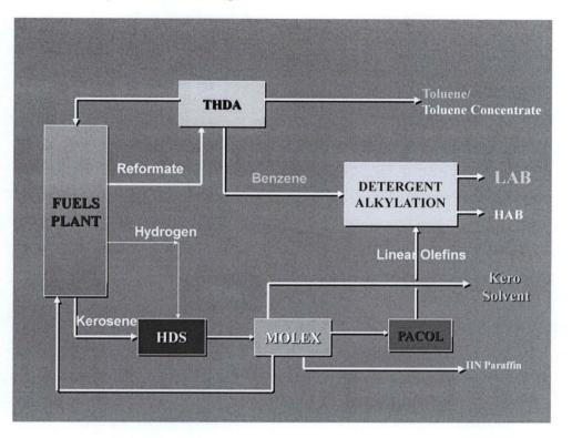
Fig. 2.5 Schematic Flow Diagram of LAB Plant. (Source: Egbe, 2008)
