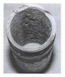
Plate x. Crevice Corrosion. (www.corrosion-club.com)
