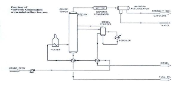
Fig.2.3 Flow Diagram of Crude Distillation Process in Refinery.
