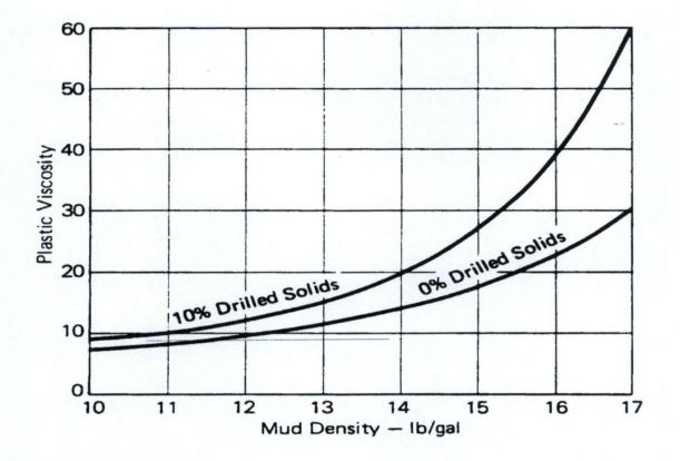
Figure 2.2: Effect of inert drilled solids on plastic viscosity.
