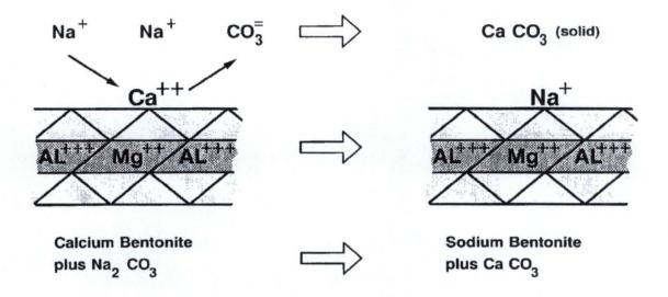
Figure 2.16: Beneficiation of Calcium Bentonite to Sodium Bentonite.
