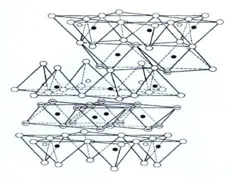
Figure 2.13: Chlorites Structure
