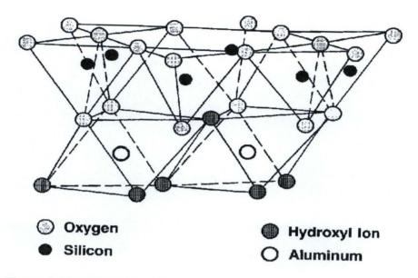
Figure 2.11: Kaolites Structure
