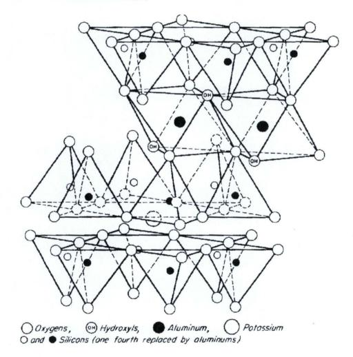
Figure 2.12: Illite Structure.
