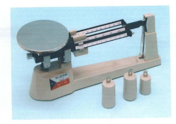
Figure 3.1 Beam Balance.
