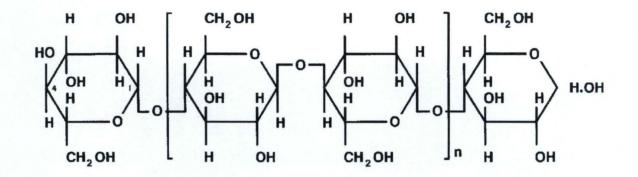
Figure 2.6: Cellulose Structure.
