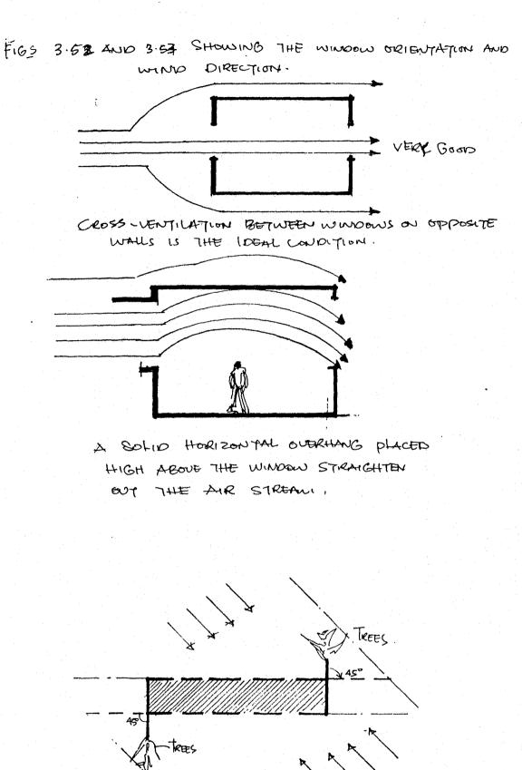
DEFLECTING WALLS AND VEGETATION CAN BEUSED TO CHANGE AIR FLOW DIRECTION SO THAT THE OPTIMUM SOLAR DRIENTATION CAN BE MAINTAINED. Usually indoor ventilation is better from oblique winds than from head-on windows, because the oblique air stream covers more of the room.
