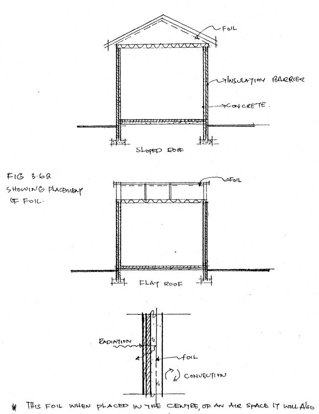
SLIGHTLY REDUCE HEAT FLOW BY CONVERTION.
