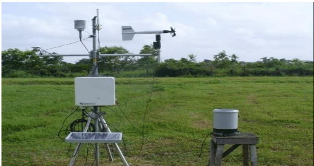
Plate I Campbell ground-based weather station with different meteorological instruments ( Source: Naipal et al. , 2013)
