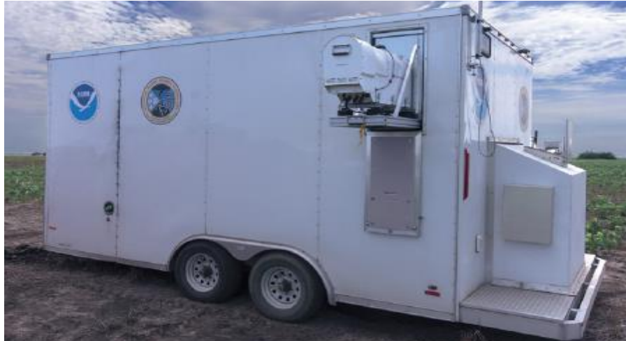
Plate II Picture of Collaborative Lower Atmosphere Profiling System (CLAMPS-2)
