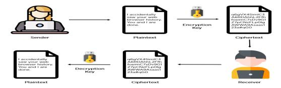
Figure 2.1: Encryption Diagram (Google, 2022)
