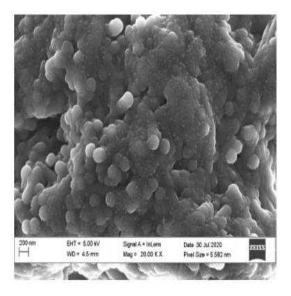
Figure 4.2: Scanning Electron Micrograph of *Eudrilus eugeniae* Aqueous Residue Fraction Mediated- Silver Nanoparticles
