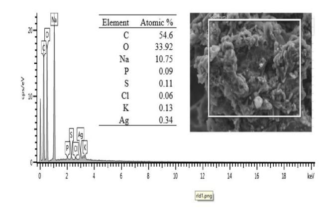
Figure 4.3: Energy Dispersive Pattern of *Eudrilus eugeniae* Aqueous Residual Fraction Mediated Silver Nanoparticle
