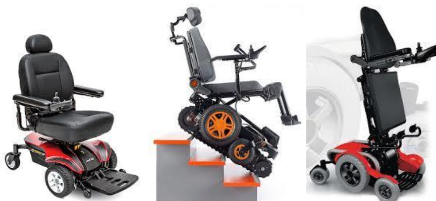
Plate III: Smart wheelchair, a stairs climbing wheelchair and a stand up wheelchair (Leaman and Hung, 2017)
