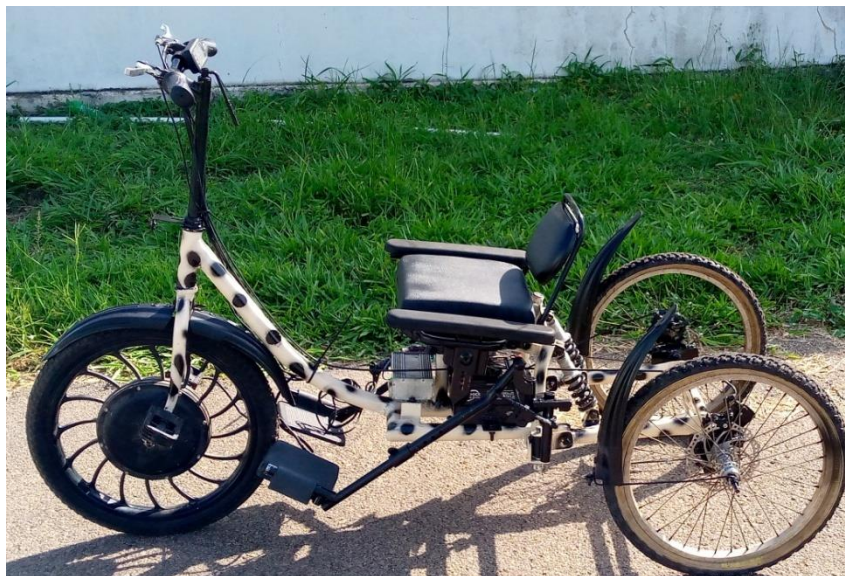
Plate XVIII: Tricycle with adjustable wheel camber developed during this project, July, 2021
