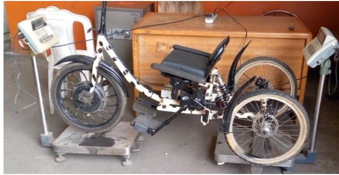
Plate IX: Axle weight measurement, July, 2021
