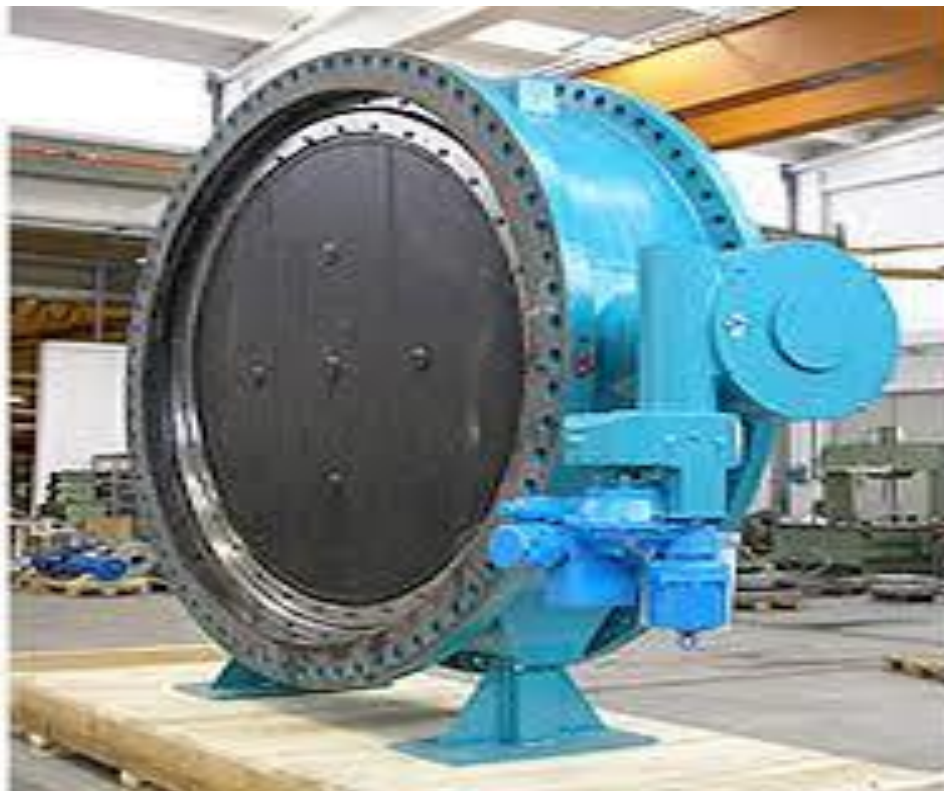
Plate III: A transmission main valve (Municipal Water Works, Minna)
