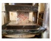
Plate 9: Plain concrete cube under Plate 10: 5% PET concrete cube under compression machine
