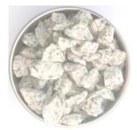
Plate II: Crushed granite stone as coarse aggregate
