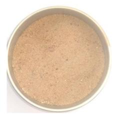
Plate III: River sand as fine aggregate
