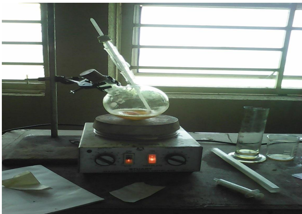
Plate III: Setup for Biolubricant Production
