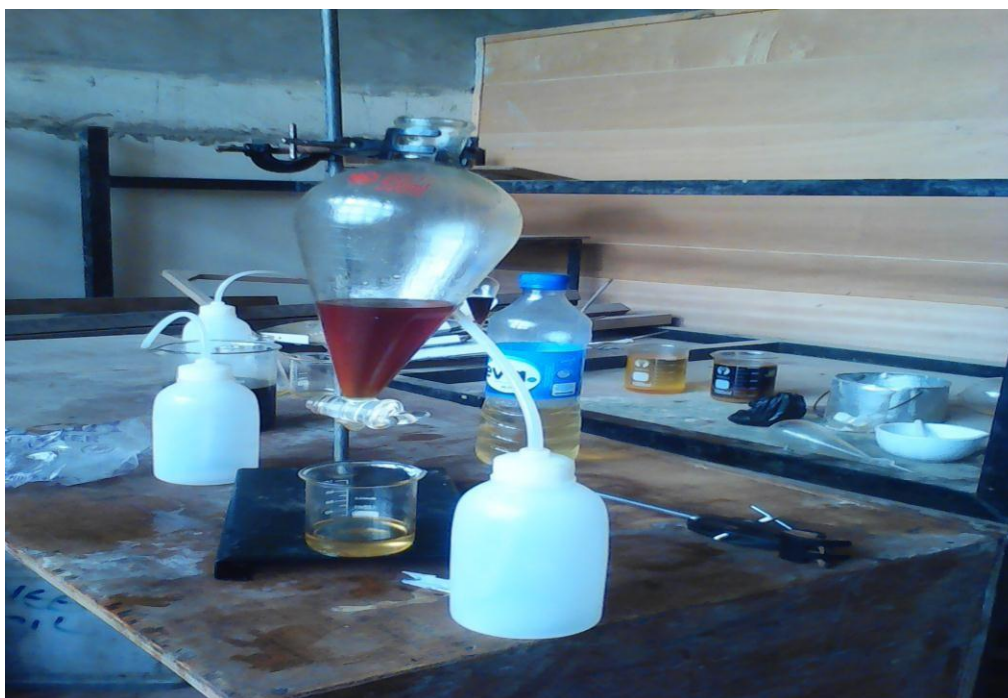
Plate IV: The Set up for the Washing of Biolubricant
