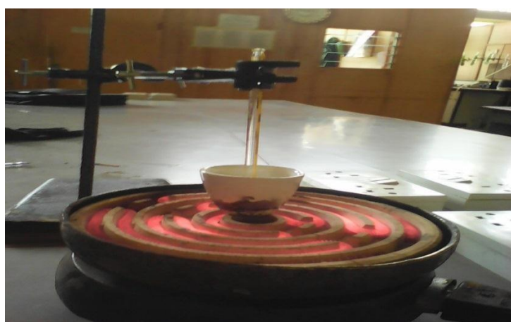
Plate V; Setup for Flash point of Biolubricant
