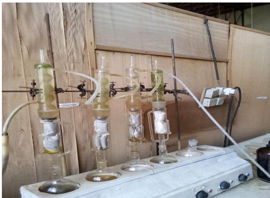
Plate II: The: Set-up of Continuous Soxhlet Apparatus for Extraction Process.
