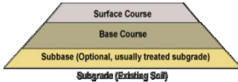
Figure 2.2: Schematic of a Flexible Pavement
