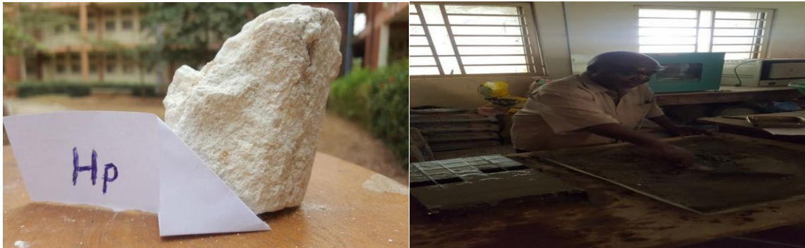
B1: Sample of High purity Metakaolin B2: Preparations of Mortar cubes and demould cubes
