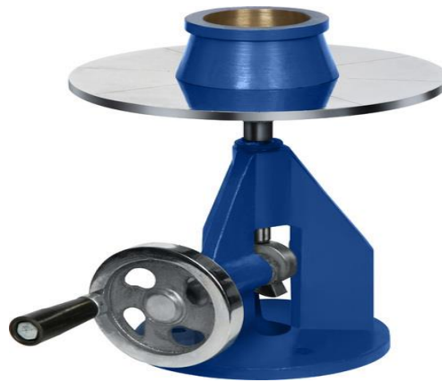
Figure 4.5 Flow table concrete test
