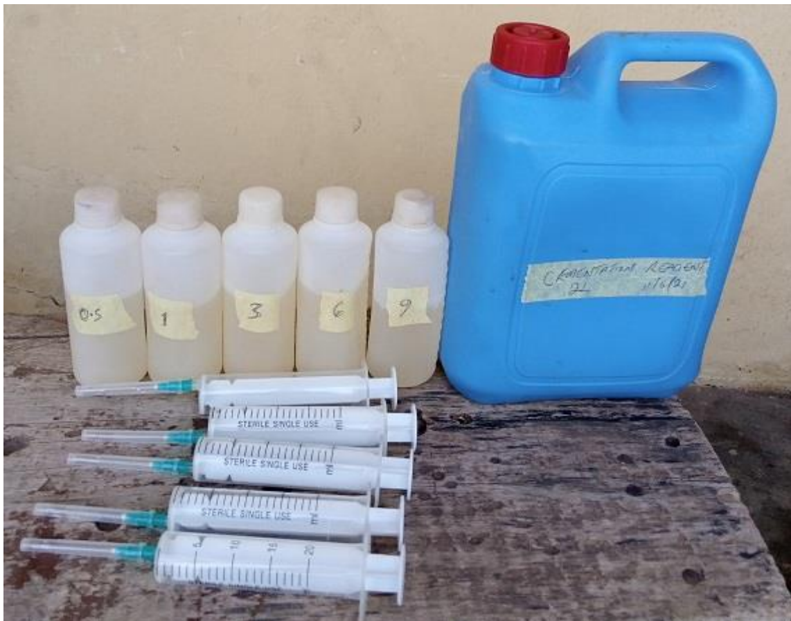
Plate VI: Bacteria and cementation reagent (MICP treatment)
