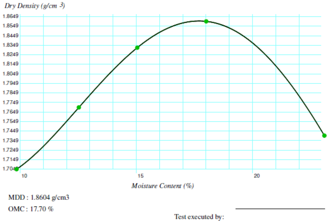
Figure C2: MDD and corresponding OMC of studied soil sample treated with 3% rock flour and 2.5% lime (BSH)
