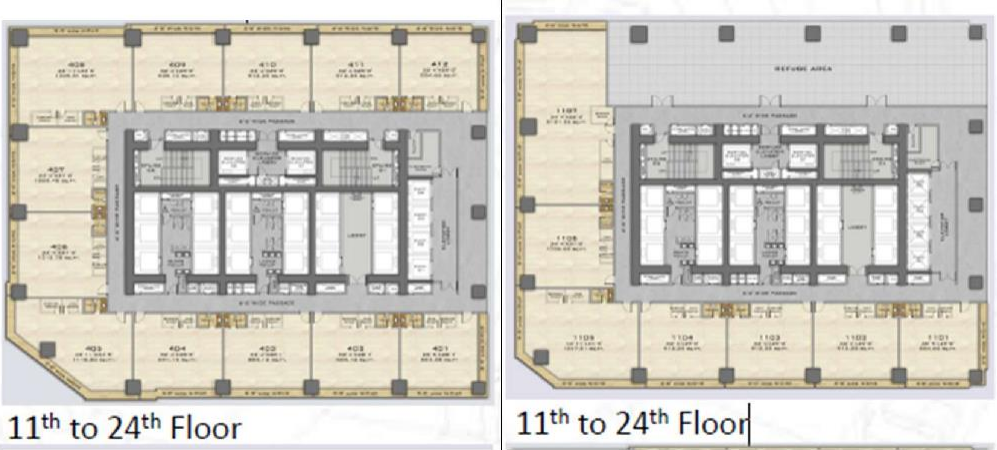
Figure 4.7: The floor plans reveal a central core system and external bearing walls
