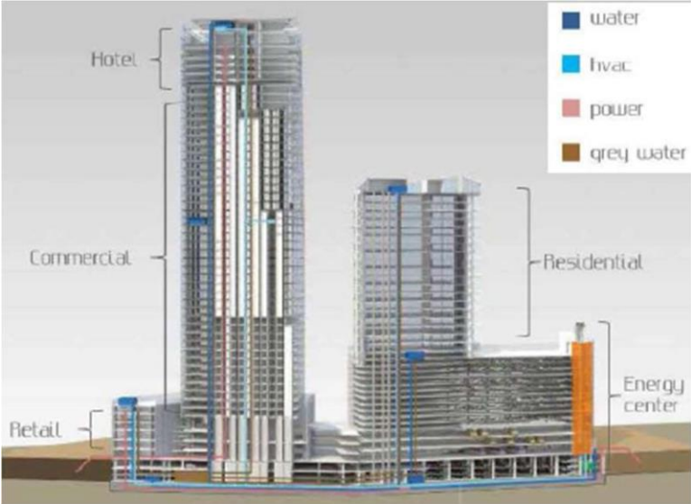
Figure 4.8: Section and zoning of the Mixed-use building
