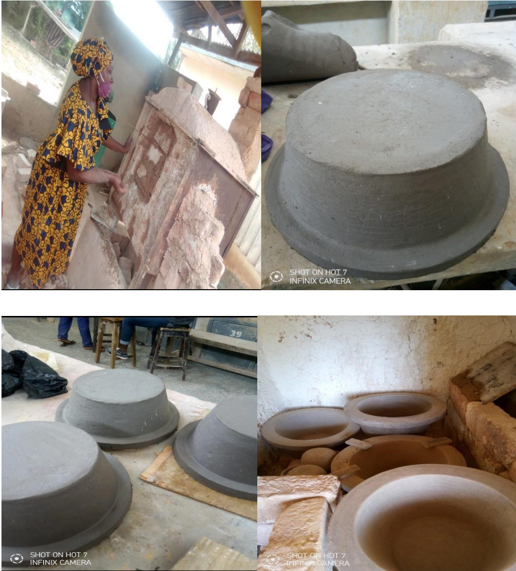
Plate E2: Fabrication process images of the filters (a) Kiln sealing (b) Greenware (c) Greenware drying (d) Sintered filters
