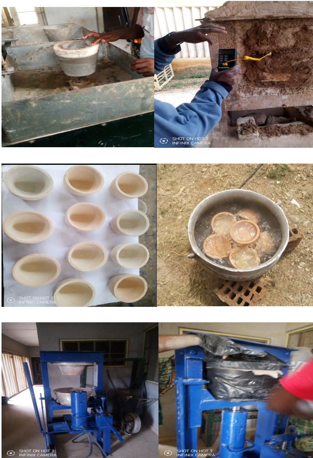
Plate E1: Fabrication process images of the filters (a) Jigle jolly moulding (b) Gas kiln sintering (c) Sintered small filters (d) Saturation process (e) The hydraulic press (e) Big filter pressing process
