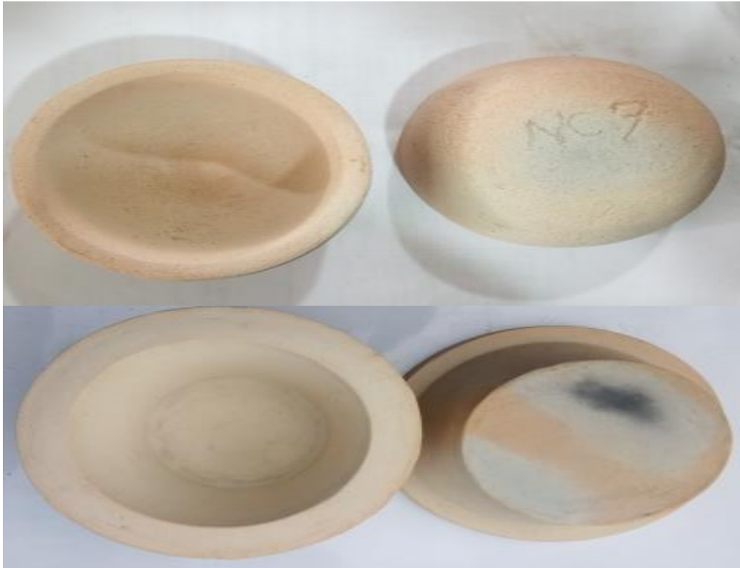
Plate XX: Fabricated small (NC7 s ) and big (NC7 B ) filters with Ag 2 O-TiO 2
