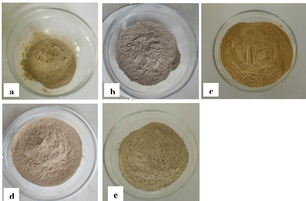
Plate VII: Nanocomposites of (a) Ag 2 O-clay, (b) TiO 2 -clay, (c) Ag 2 O/TiO 2 (75%)-clay (25%), (d) Ag 2 O/TiO 2 (50%)-clay (50%), and (e) Ag 2 O/TiO 2 (25%)-clay (75%)
