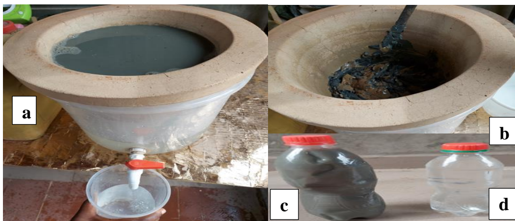
Plate VIII: Pictorial representation of (a) Assembled filter for the wastewater treatment, (b) residue, (c) mining wastewater, and (d) treated mining water
