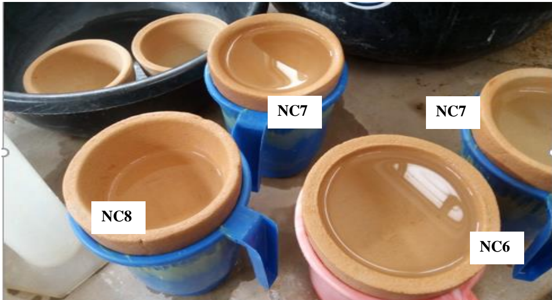
Plate XIX: Flowrate test of ceramic filters of (a) NC6, (b) NC7 and (c) NC8
