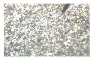
**Plate 1:** Microstructure of the mild steel before heat treatment  $\times$  400; Ferrite (Whitish) and iron carbide (Fe<sub>3</sub>C) phases clearly shown in an intermixed assemblage.
