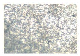
**Plate 7:** Micro graphs after case hardening with the mixture of charcoal and sea shells at 950 <sup>0</sup>C at magnifications of 600, and two hours soaking time. Ferrite transformation also favoured with finer grains.
