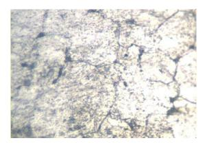
**Plate 3:** Micro graph after case hardening with charcoal at 900 <sup>0</sup>C at magnification of 600, and three hours soaking time. Transformation of Ferrite to iron carbide was favoured by significant uptake of more carbon from the charcoal.
