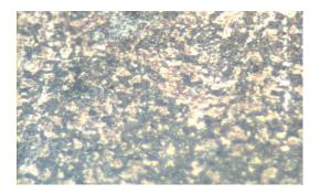
**Plate 5:** Micro graphs after case hardening with sea shells at 950 <sup>0</sup>C at magnification of 600, and holding time of two hours. Ferrite grains with interstitial carbide.
