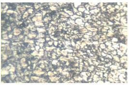
**Plate 6**: Micrographs after case hardening with the mixture of animal bone, charcoal and sea Shells at 950 <sup>0</sup>C at magnification of 600, and two hours soaking time. Finer grains with few transformation from ferrite to iron carbide favoured by carbon uptake.
