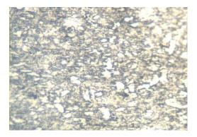
**Plate 2:** Micro graph after case hardening with animal bone at 950 <sup>0</sup>C at magnification of 600, and two hours soaking time. Ferrite is still distinctly seen untransformed.
