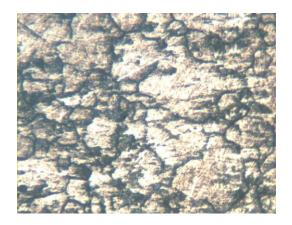
**Plate 4:** Micro graphs after case hardening with sea shells at 900  $^{0}$ C ×600, and holding time of three hours. Coarser grains of Ferrite with interstitial iron carbide.
