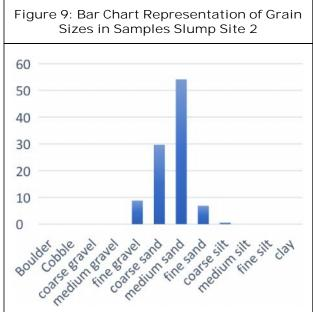
fine sand, coarse silt and fine gravel. Estimated values of  $C_u$  and  $C_c$  are 0.57 and 0.148 respectively, which indicates it is poorly graded. Table 5 is the sieve analysis result for slump site 3.
