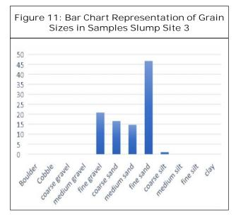
the sample contains high amounts of fine sand, medium to coarse sand and fine gravel. Estimated values of  $C_u$  and  $C_c$  are 5.31 and 0.711 respectively. The  $C_u$  reflects substantial amount of gravel, and is fairly graded.
