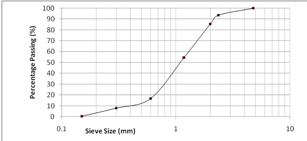
Figure 1.0: Particle size distribution of sand used
