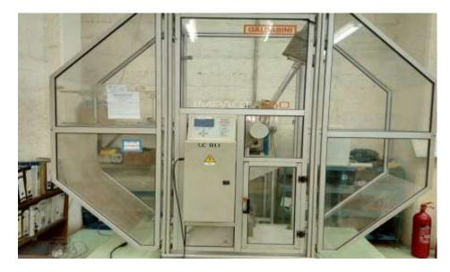
**Plate VII: Impact testing machine**
