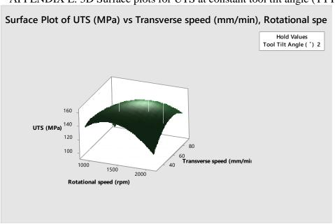
APPENDIX L: 3D Surface plots for UTS at constant tool tilt angle (TTT)
