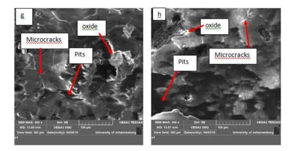
Plate XIX (b) : Magnification at 500X for (e) optimal weldment TT15 (f) optimal weldment TTT15 (g) corroded optimal TT15 (h) corroded optimal TTT15
