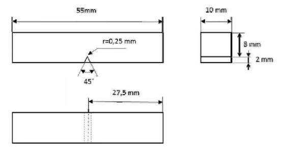
**Figure 3.6: Impact specimen dimensions**
