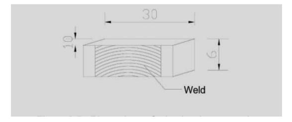
Figure 3.4 Dimensions of microhardness specimen in mm
