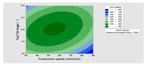
Figure 4.38: Contour plot for UTS at constant rotational speed
