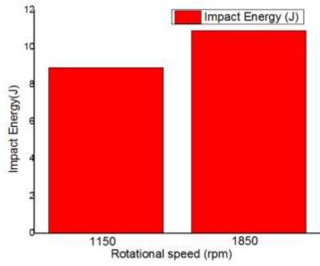
Figure 4.10: Impact energy at varying rotational speed
