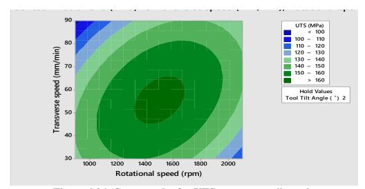
Figure 4.36: Contour plot for UTS at constant tilt angle
