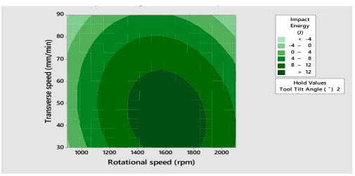
Figure 4.29: Contour plot for impact energy at constant tilt angle
