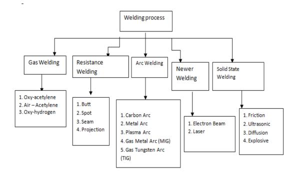
Figure 2.1: Classification of Welding processes (Tri-state fabricators, 2010)
