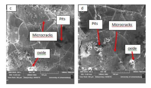
Plate XIX (a): Magnification at 500X for (a) AA7075 (b) 1200 (c) corroded AA7075 (d) corroded AA1200
