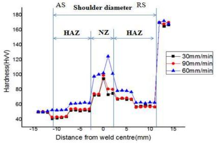
Figure 4.12: Hardness profile for tapered threaded tool
