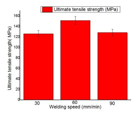
Figure 4.6: UTS at varying welding speed
