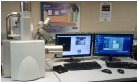
Plate IX: Scanning Electron Microscope
