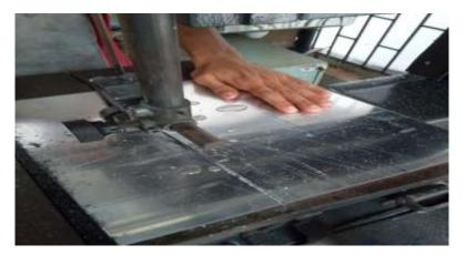
Plate XI: Cutting of workpiece using band saw
