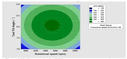
Figure 4.37: Contour plot for UTS at constant transverse speed
