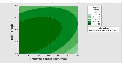
Figure 4.31: Contour plots for impact energy at constant rotational speed
