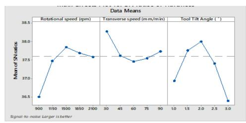
Figure 4.42: Main effects plot for signal to noise ratios (S/N) of hardness
