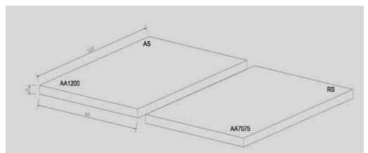
Figure 3.1: Dimensions of work piece material
