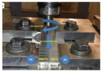
Plate I: Experimental welding configuration Source: (Paradiso *et al.* 2017)
