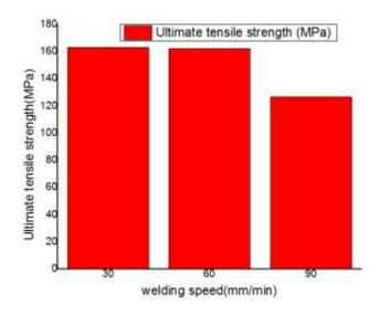
Figure 4.16: UTS at varying welding speed
