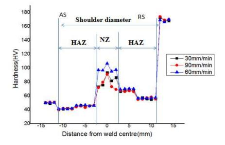
Figure 4.2: Hardness profile at different welding speed for TT
