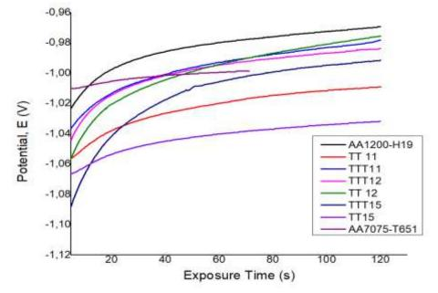
Figure 4.50: OCP versus exposure time
