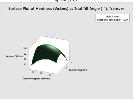
APPENDIX D: 3D Surface plots for hardness at constant rotational speed (TT)
