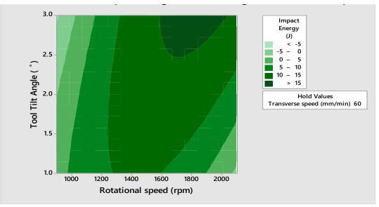
Figure 4.40: Contour for impact energy at constant transverse speed
