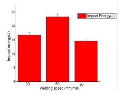
Figure 4.19: Impact energy at varying weld speed
