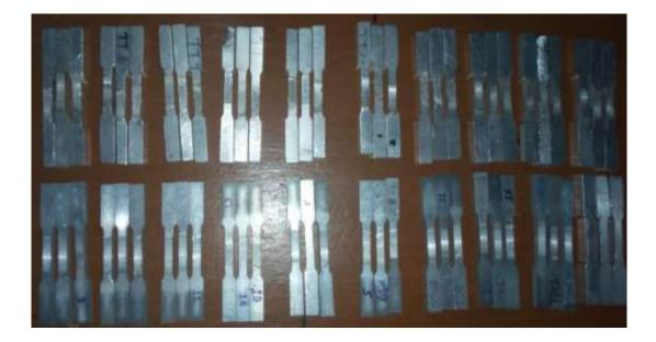
**Plate XIV: Tensile test specimens**
