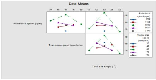
Figure 4.22: Interaction plot for hardness (Vickers)
