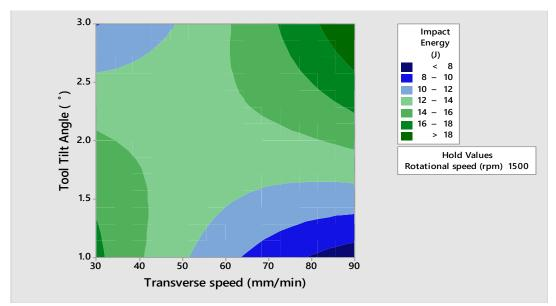
**Figure 4.41: Contour plot for impact energy at constant rotational speed** The contour plot indicates how change in tool tilt angle (°) and tool rotational speed (rpm) affects the impact energy of the weldment while keeping transverse speed (mm/min) constant at 60 mm/min. The result indicates that impact energy values of 16-18 J can be achieved using tilt angle of 2.5 ° and TS of 90 mm/min.
