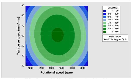
Figure 4.26: Contour plot for UTS at constant tilt angle
