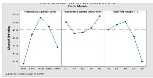
Figure 4.43: Main effect plot for signal to noise ratios (S/N) of UTS
