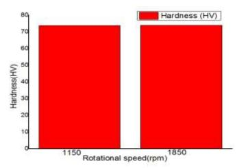
**Figure 4.4: Hardness at varying rotational**
