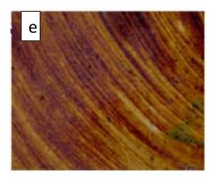
Plate XX: Optical images of material flow pattern and microstructure of nugget zone of tapered tool optimal weldment at 100X magnification: (a) Micrograph of joint, (b) material flow pattern, (c) unmixed, (d) mechanically mixed, (e) mixed region, (j) joint interface
