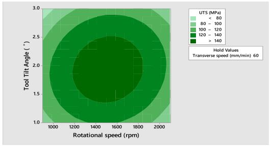
Contour plot for UTS at constant transverse speed is shown in Figure 4.27.
