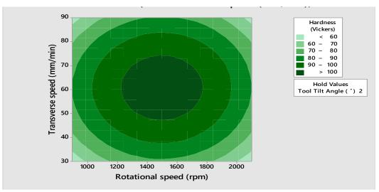
Figure 4.33: Contour plot for hardness at constant tilt angle
