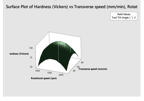
APPENDIX I: 3d surface plots for hardness at constant tool tilt angle (TTT)
