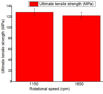
Figure 4.7: UTS at varying rotational speed
