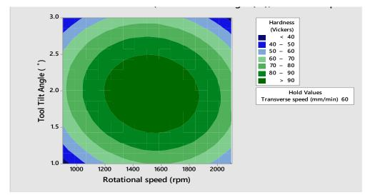
Figure 4.24: Contour plot for hardness at constant traverse speed
