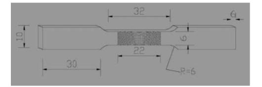
**Figure 3.5: Tensile specimen dimensions**
