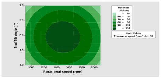
Figure 4.34: Contour plot for hardness at constant transverse speed
