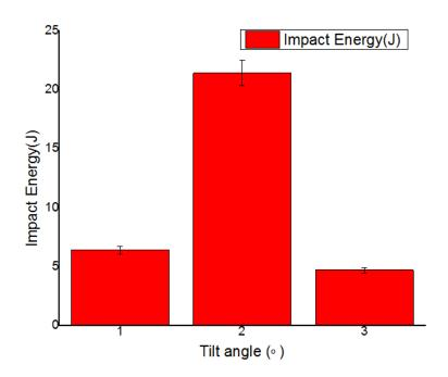
Figure 4.11: Effect of tilt angle on impact energy
