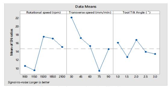
Figure 4.47: Main effect plot for signal to noise ratios (S/N) of impact energy
