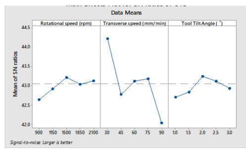
Figure 4.46: Main effect plot for signal to noise ratios (S/N) of UTS
