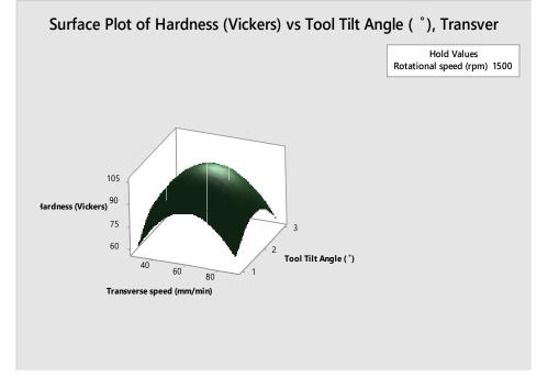
APPENDIX K: 3D Surface plots for hardness at constant rotational speed (TTT)
