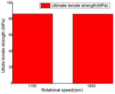
Figure 4.17: UTS at varying rotational speed
