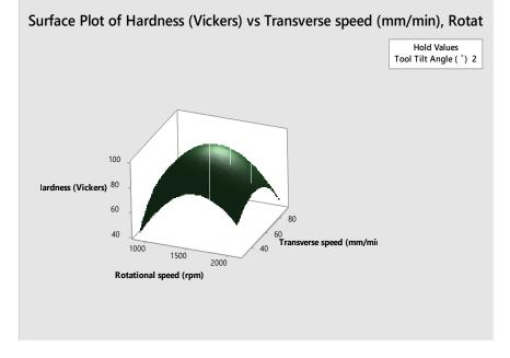
APPENDIX B: 3D Surface plots for hardness at constant tilt angle (TT)
