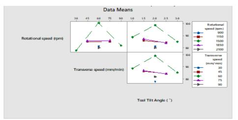
Figure 4.32: Interaction plot for hardness (Vickers)
