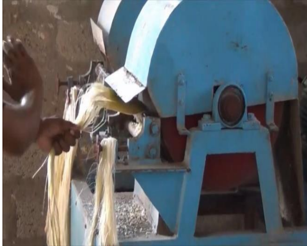
Plate I11: Banana Fiber Extracting Machine (Rahamatthulla et al. , 2018).
