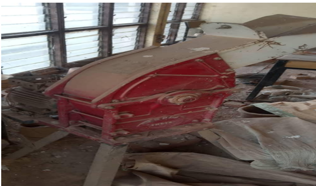
Plate II: Hammer mill machine (Spectral Laboratory Services, Tudun-wada, Kaduna)
