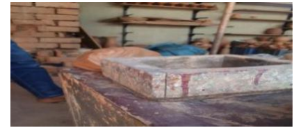
Plate VI: Forming of brick in mould
