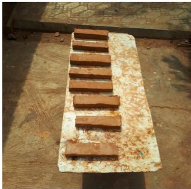
Plate VII: Sun drying of some brick samples produced
