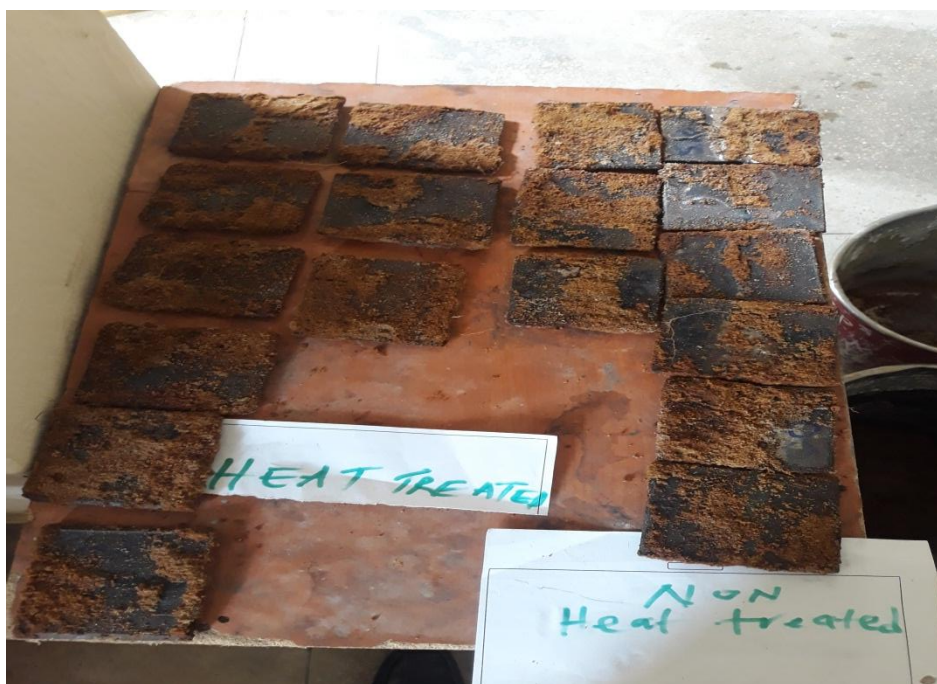
Plate XVIII: Typical corroded Samples
