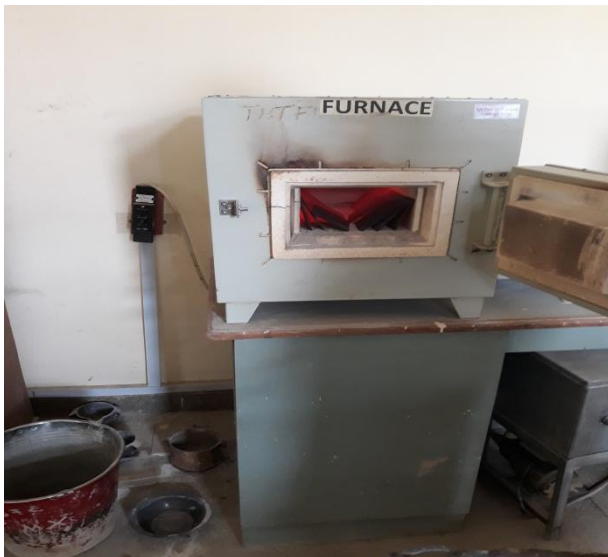
Plate VII: Heated samples in the furnace
