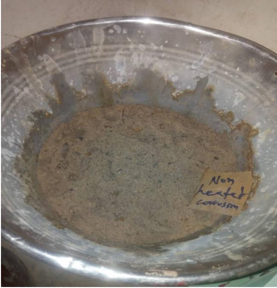
Plate XII: Soil bath for non-heat treated
