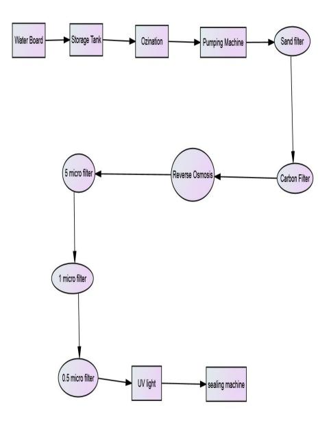
Figure D5: Table Water E production processes
