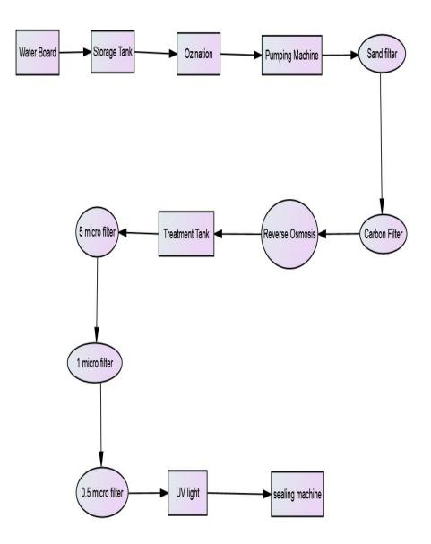
Figure D2: Table Water B production processes
