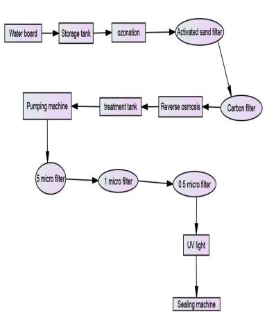
Figure D1: Table Water A production processes
