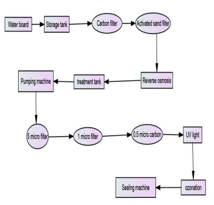
Figure D3: Table Water C production processes
