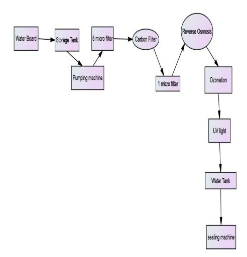
Figure D4: Table Water D production processes
