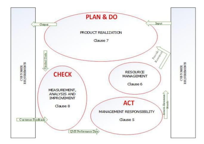
Figure 2.2: Process-based Approach to Quality Management
