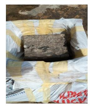
Plate I: Concrete Curing Mould
