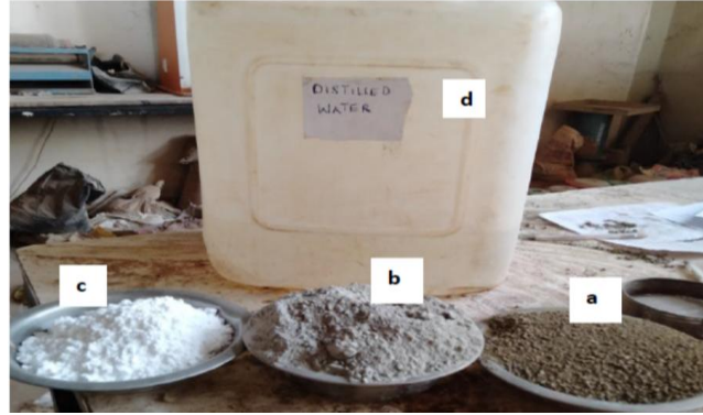
Figure 3.1: Materials used in the study: (a) Tropical Black clay, (b) cement, (c) zeolite, (d) distilled water, used for this study
