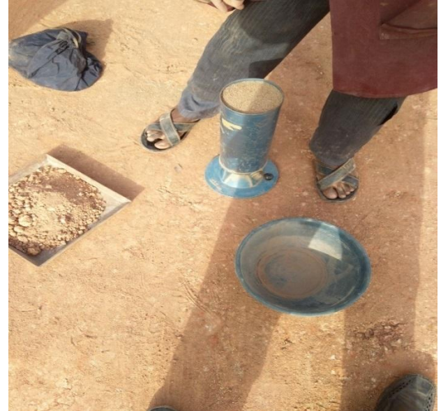
Plate VIII: In-situ density test on compacted finished surface.
