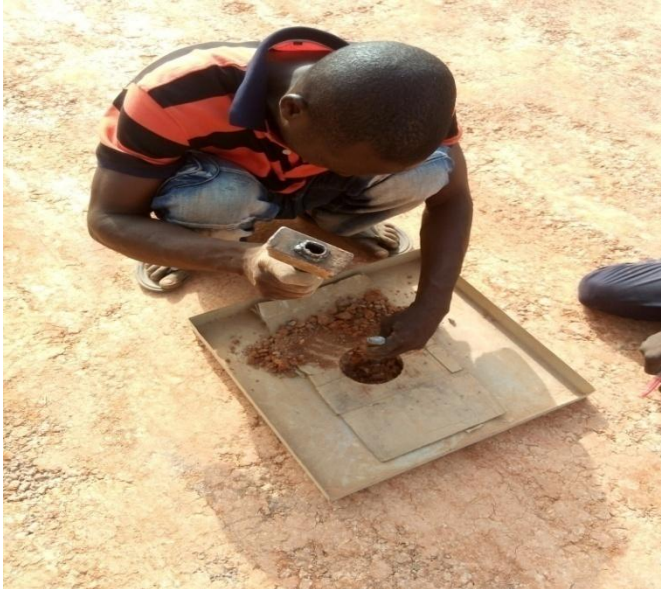
Plate VIII: In-situ density test on compacted finished surface.
