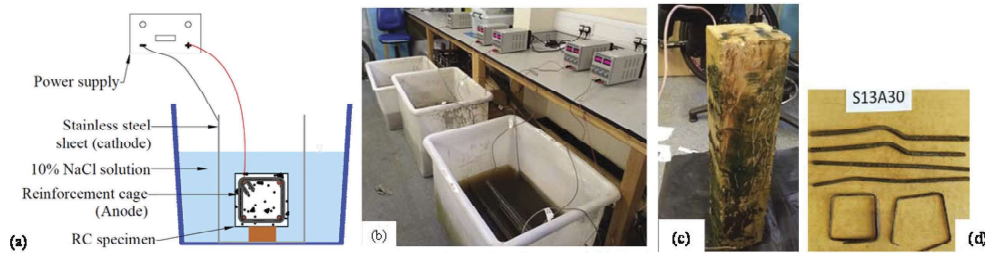
Figure 1. Accelerated corrosion procedure; (a) Schematic setup drawing, (b) laboratory setup (c) corroded columns after completion of corrosion and (d) corroded rebars after cleaning.
