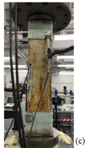
Figure 3. Experimental test setup (a) laboratory setup; (b) schematic of the LVDT connection; (c) Image of the LVDT connections to the RC samples.
