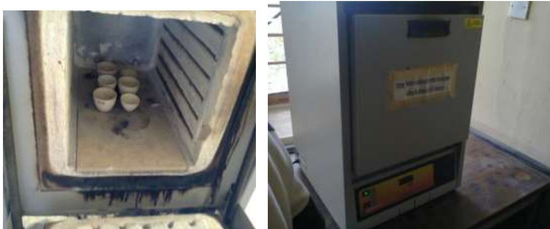
Plate II: Muffle Furnace (Model No: HZ-1733A) used for ash content determination
