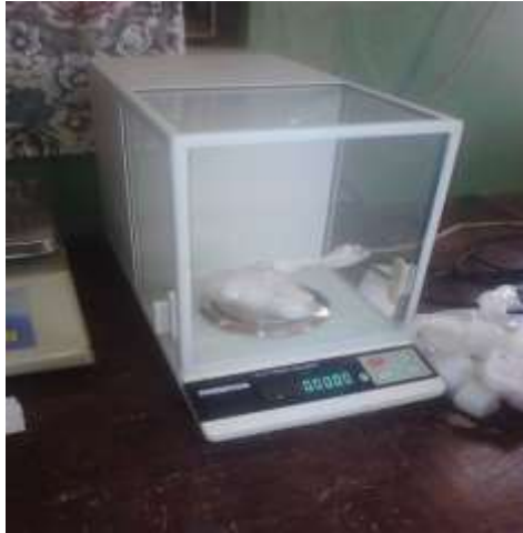
Plate III: Electronic weight balance (Model No: XY-Q50B).
