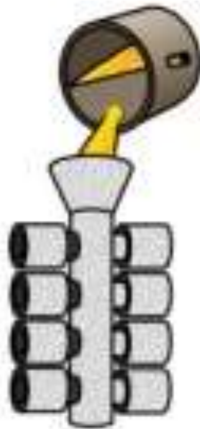
Figure 2.5: Pouring of molten metal into the mould
