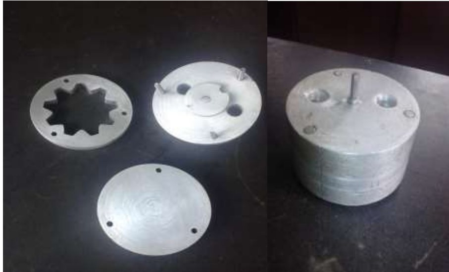
Plate IV: Components and assembling of wax pattern die
