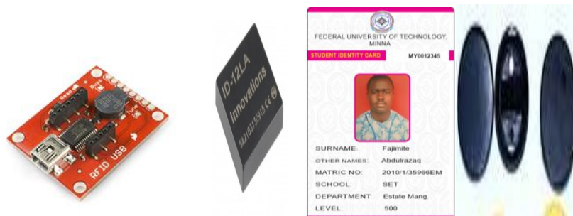
Figure 4: RFID reader module and tags (adapted from [12])
