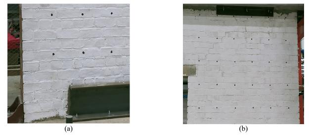
Figure 4. Failure modes of URM at different displacement loading. (a) Lateral crack at the base at 3mm (b) diagonal cracks at the edge of window opening towards the top at 4mm
