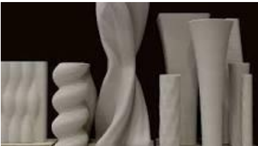
Figure 11: Concrete Elements Produced via 3D Concrete Printing
