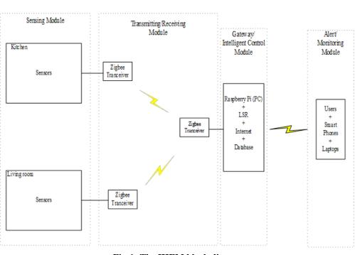
Fig-1: The IHEM block diagram
