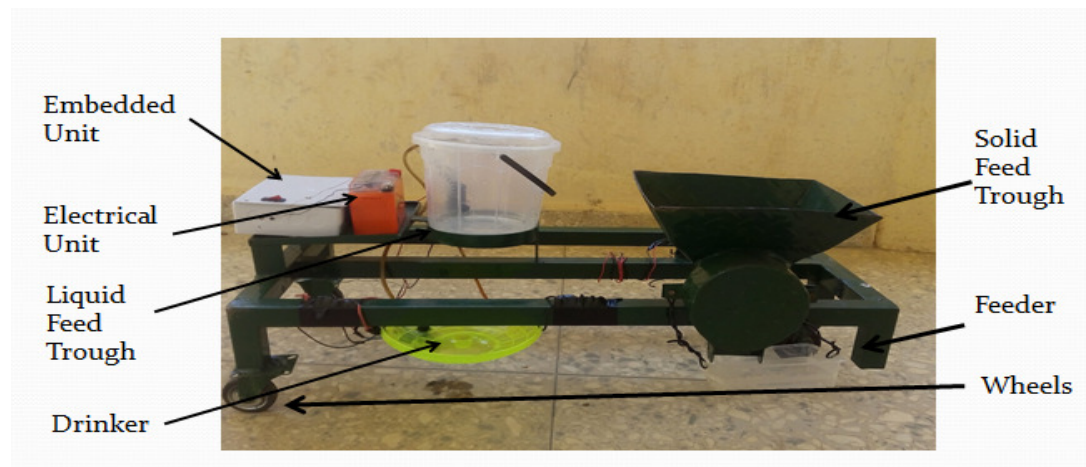
Figure 6: Overview of the developed mobile intelligent poultry feed dispensing system The performance of the system using the PSO tuned PID controller was evaluated in terms of the rise time, settling time and overshoot. Figure 8 and 9 show the system response of the liquid and solid feed dispensing units respectively.
