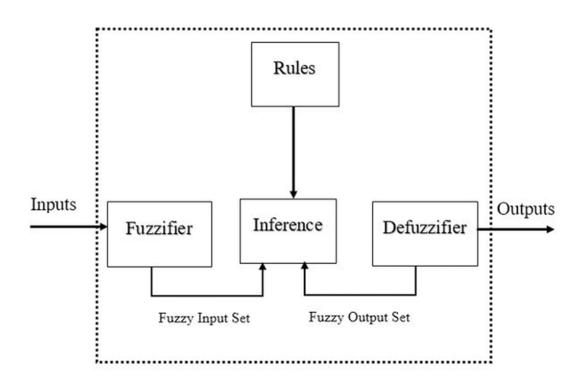
Fuzzification is the process of converting a crisp input into a fuzzy input (Olaniyi et al., 2014). This is usually achieved using membership functions. A membership function is a graphical representation of how a crisp input is mapped to a degree of membership from 0 to 1 (Waris & Ahmad, 2011). There are different types of membership functions used in fuzzy logic, which include triangular, trapezoidal, Gaussian and singleton membership functions (Goni, Gumpy, & Zira, 2018).
