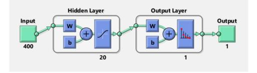
The inputs to the ANN are the SURF features, while the output is the classification result. The neural network was designed using a 70-15-15 rule. This means that 70% of the data was used for training, 15% for testing, and 15% for validation. The network was evaluated using the Receiver Operating Characteristic (ROC) which is a metric for evaluation of classification performance. Figure 11 shows the ROC curve for the ANN.
