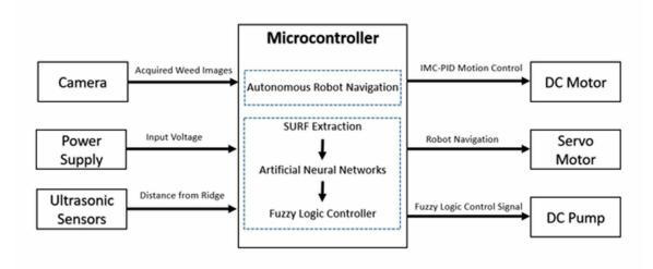
Figure 3. Circuit Diagram of Mobile Robot
