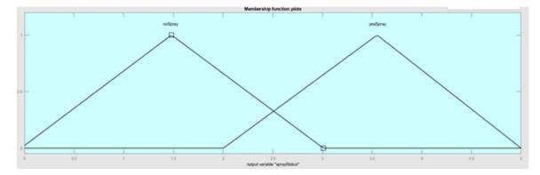
The input to the FIS is the presence or absence of weed. This parameter is obtained from the output of the neural network. The input consists of two membership functions. These functions are noWeed and yesWeed with ranges of -0.5 to 0.72 and 0.14 to 1.5, respectively. The output of the FIS is the application of the herbicide. The output consists of two membership functions which are noSpray and yesSpray with ranges of -0.03 to 3.0 and 2.0 to 5.0 respectively.
