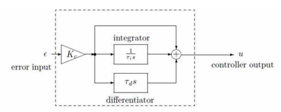
Due to the advantages exhibited by the PID controller, in this study, a PID tuning approach is adopted to ensure optimum system response, stability, and accuracy of the robot navigation. In order to implement the PID control scheme, a mathematical representation of the system must be acquired. In the case of this system, the major components are the DC motor, servo motor, and DC pump. These components can be modeled using the transfer function of an electromechanical system given in equation 2.
