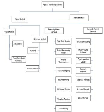
Fig 2: Classification of Pipeline Monitoring System
