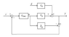
Figure 2: An IMC Control Process [6]
