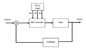
Figure 5: FL-PID Control System
