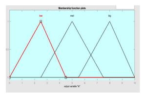
Figure 7: Membership Function for Change in Input
