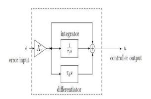
Figure 1: A PID Control Process [19].
