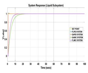
Figure 24: System Response of Liquid Subsystem
