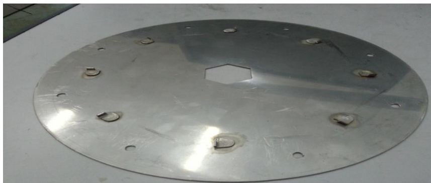
Figure 2. Eight holes seed plate
