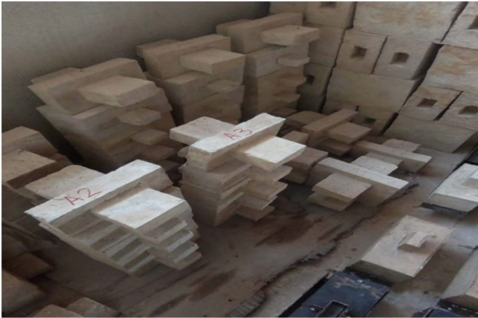
Fig. 2. Freshly demolded clay brick components
