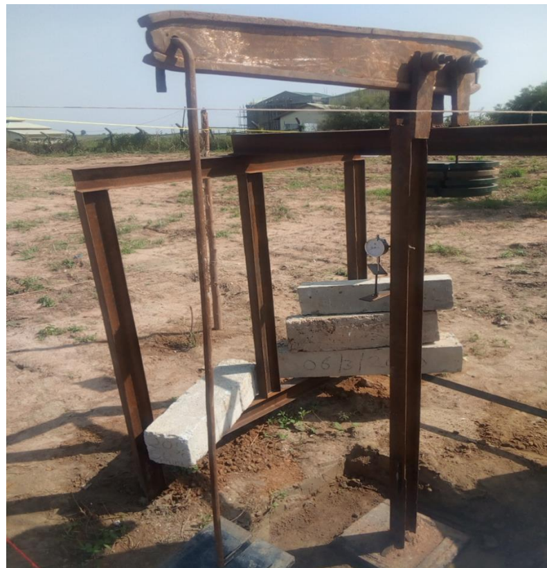
Figure 6. Proposed Set-up for Innovative Field Plate Load Test.
