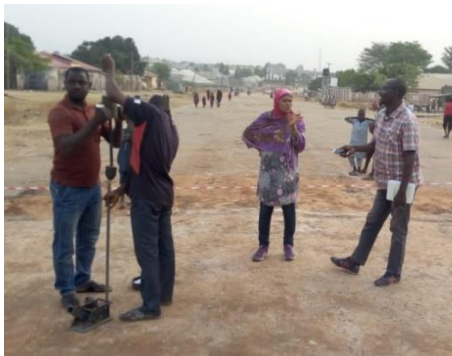
Fig. 6: Dynamic cone penetration test to estimate CBR of the test sections
